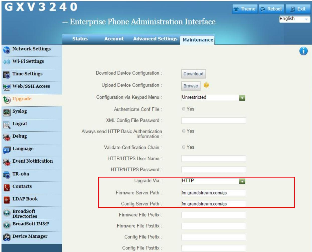
Figure 17: Upload GXV3240 Firmware via Web GUI
