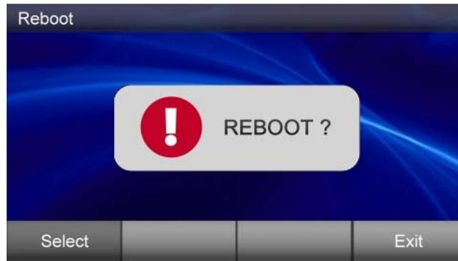
**Note:** The IP3072 takes about 2 minutes to startup after rebooting; there will be a series of diagnostic lights on the phone during the process. If your phone does not become operational within 2 minutes, contact your administrator or Service Provider support line.
