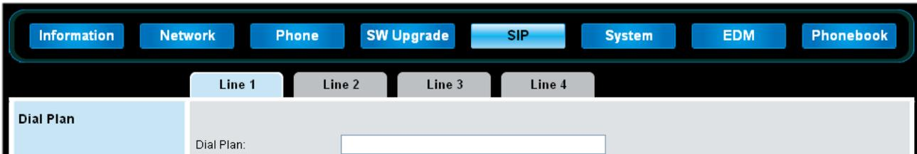
A dial plan is a set of rules for determining whether a complete set of numbers has been entered. IP3062 uses industry-standard Regular expressions to match dialed numbers.
