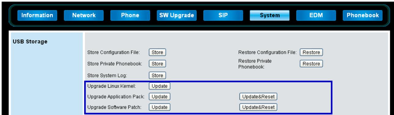
3. Press “Update” button, and then the phone will get the firmware from the USB memory dongle and start upgrading; or press “Update&Reset” button, and then the phone will do firmware upgrade and reset configuration file to default.
